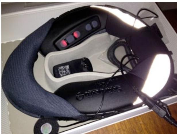
*The SRC is unique in that it's built right into the collar. All the controls are glove-friendly and located on the left side of the collar to keep your throttle/brake hand free at all times.*
