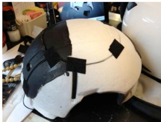
The new, longer antenna in the S2 and C3 Pro helmets fits into grooves built right into the exterior of the EPS. The antenna then plugs into the SRC and gets tucked under the lining of the helmet.
