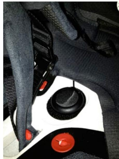
*Installing the SRC is easier if you remove the cheekpads and helmet liner, both of which snap right back in once you're done. The speakers go into an oval cutout on either side of the helmet's EPS liner and have a small range of adjustability for comfort.*
